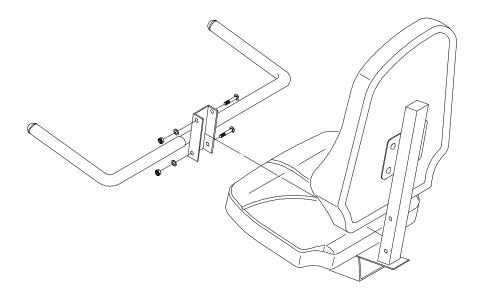
Attach handlebar to seat support bracket using: Qty 2 - (53) Button Head Screw Qty 2 - (39) Flat Washer
